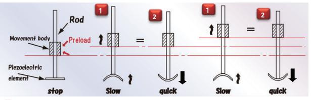
When a piezoelectric element turns in an upper direction, I turn slowly and move a shaft and a moving body together.
